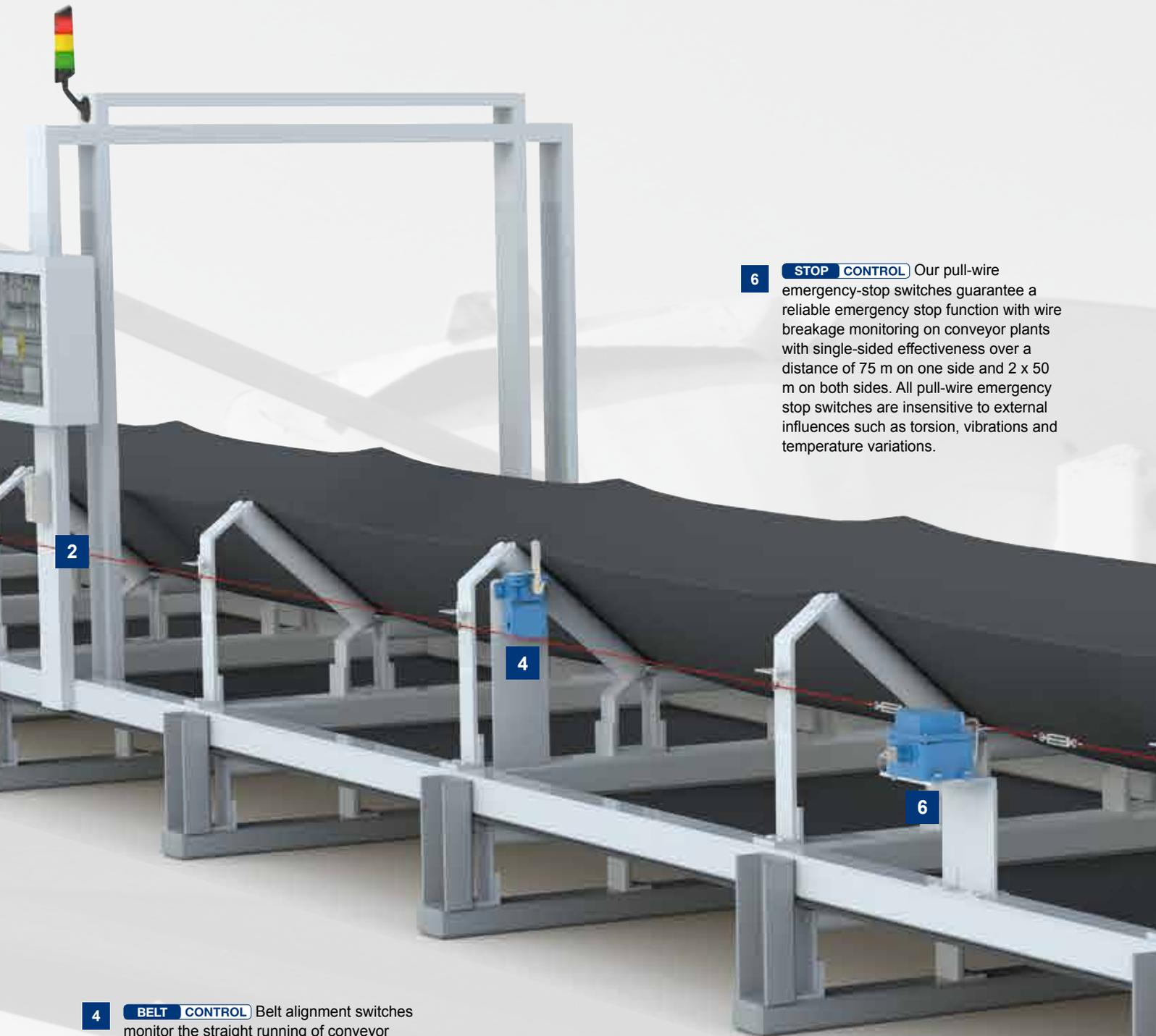
**6 STOP CONTROL** Our pull-wire emergency-stop switches guarantee a reliable emergency stop function with wire breakage monitoring on conveyor plants with single-sided effectiveness over a distance of 75 m on one side and 2 x 50 m on both sides. All pull-wire emergency stop switches are insensitive to external influences such as torsion, vibrations and temperature variations.
